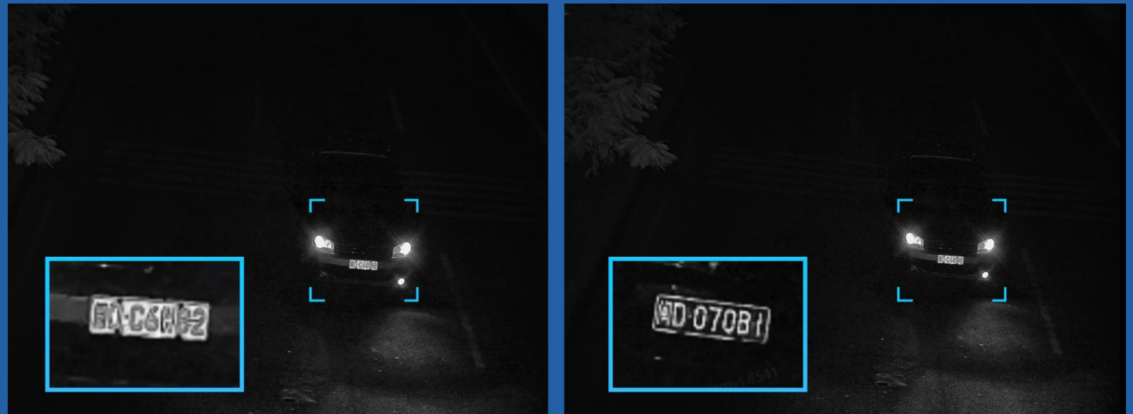
740nm IR wavelength: Ideal for low-contrast license plate recognition.
