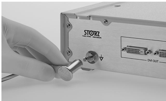
3. Connect the potential equalization cable to the outlet in the treatment room.
