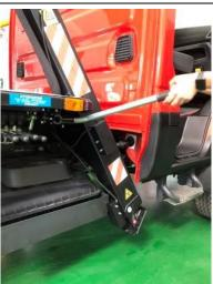
Configure the machine in transport conditions through the **(H)** stabilization controls.
