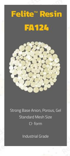
Felite™ FA124 is a highly porous, gel, Type I, strong base anion resin, supplied in the chloride form as moist, tough, uniform spherical beads. It has greater porosity, and this provides superior regeneration efficiency, easier separation in regenerable mixed beds, and greater resistance to organic fouling.
