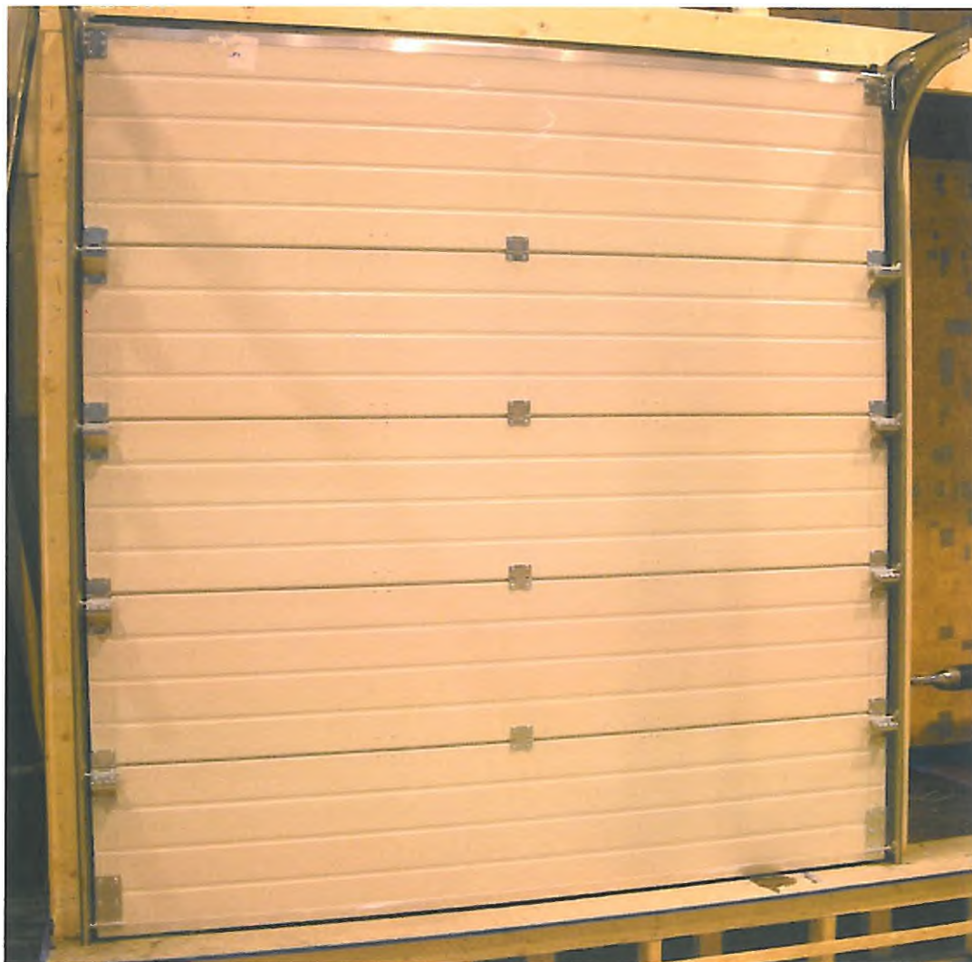
Figure 2. Door type FlexiForce RES X with Sicom panels mounted in the test rig, as seen from inside.
