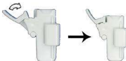
Figure 11-25. Locking the Needle Clip
