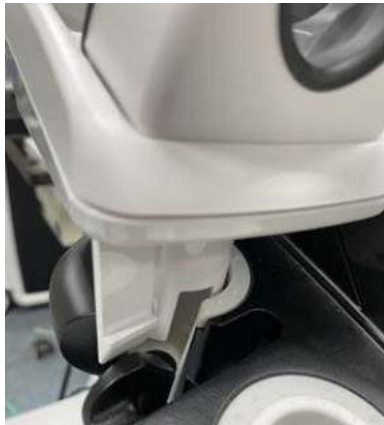
Figure 3-3. Install TVTR Probe holder
