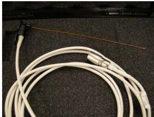
Figure 13-151. Needle Tip Sensor and Cable Close-up
