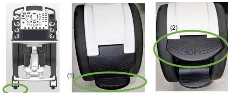
Figure 3-45. Rear-left with Swivel lock
