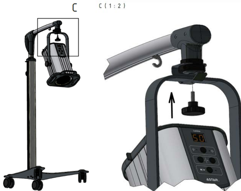
Figure 6.3. Assembly of a lamp tube to the stan
