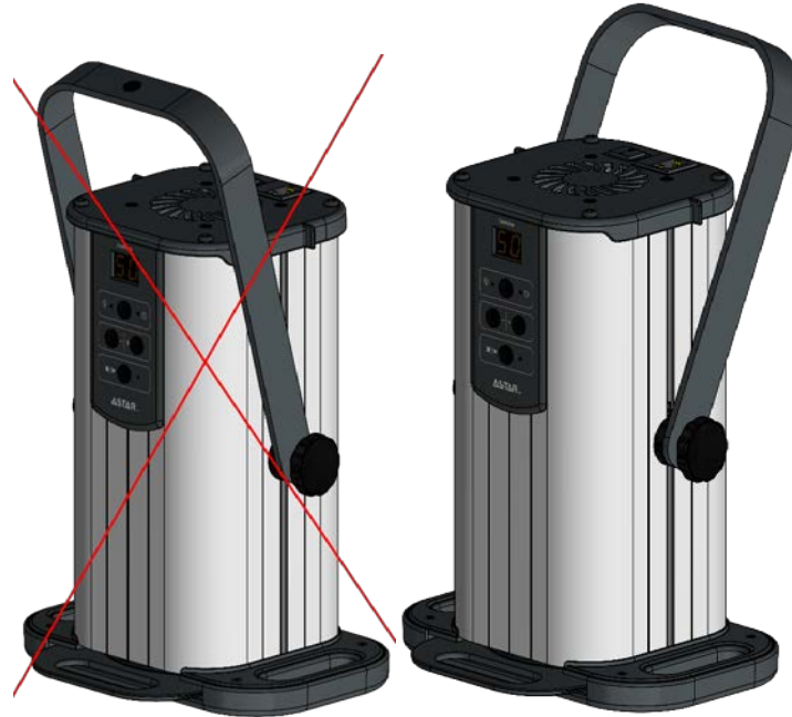
Figure 6.5. Correct position of the U-shaped holder mounted to the base
