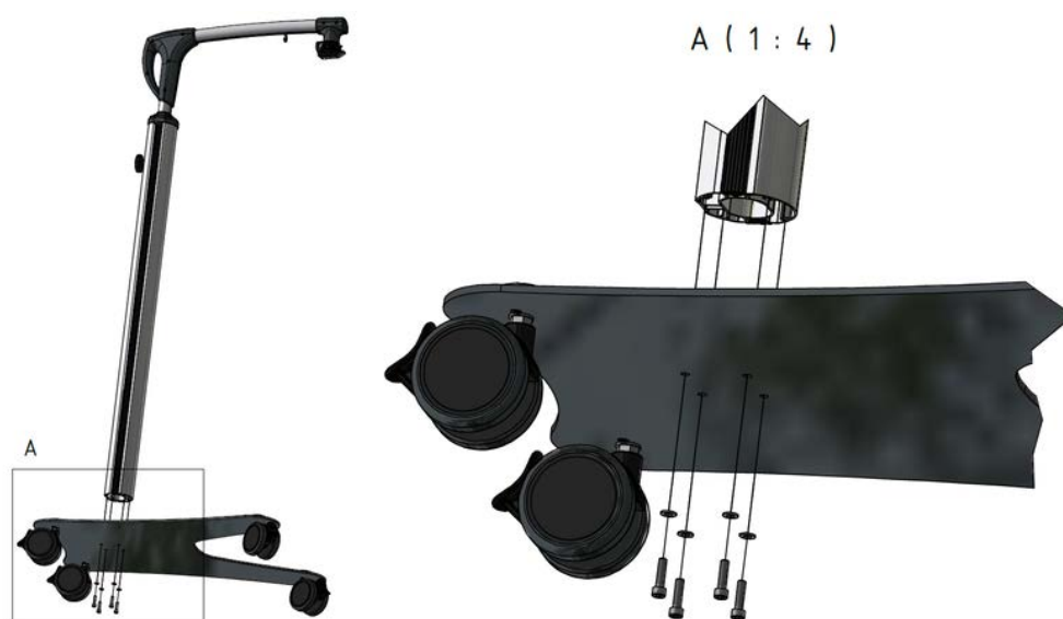
Figure 6.1. Assembly of a stand to the base
