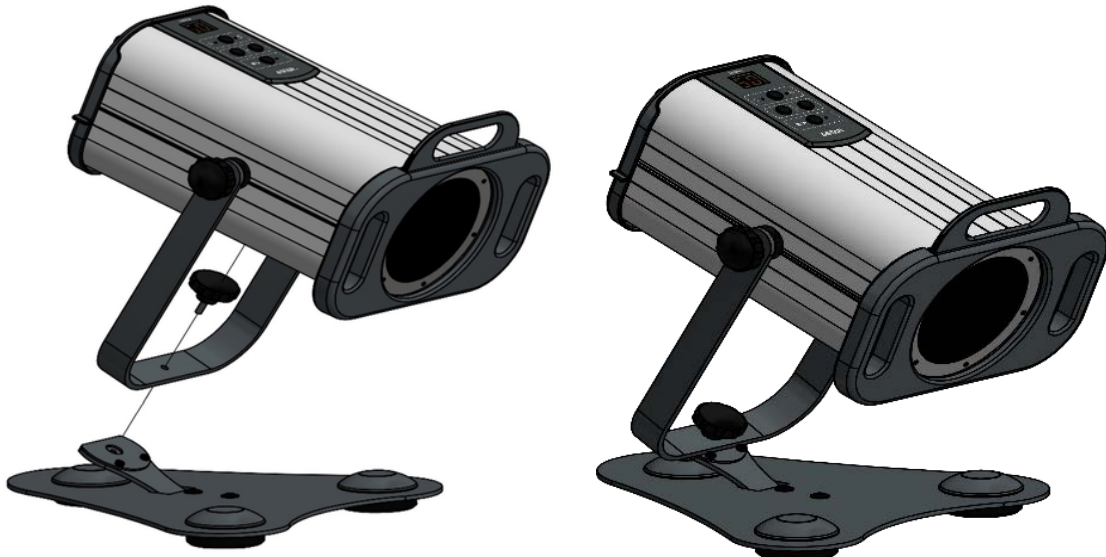
Figure 6.6. Positioning of the bushing, U-shaped holder and knob.
