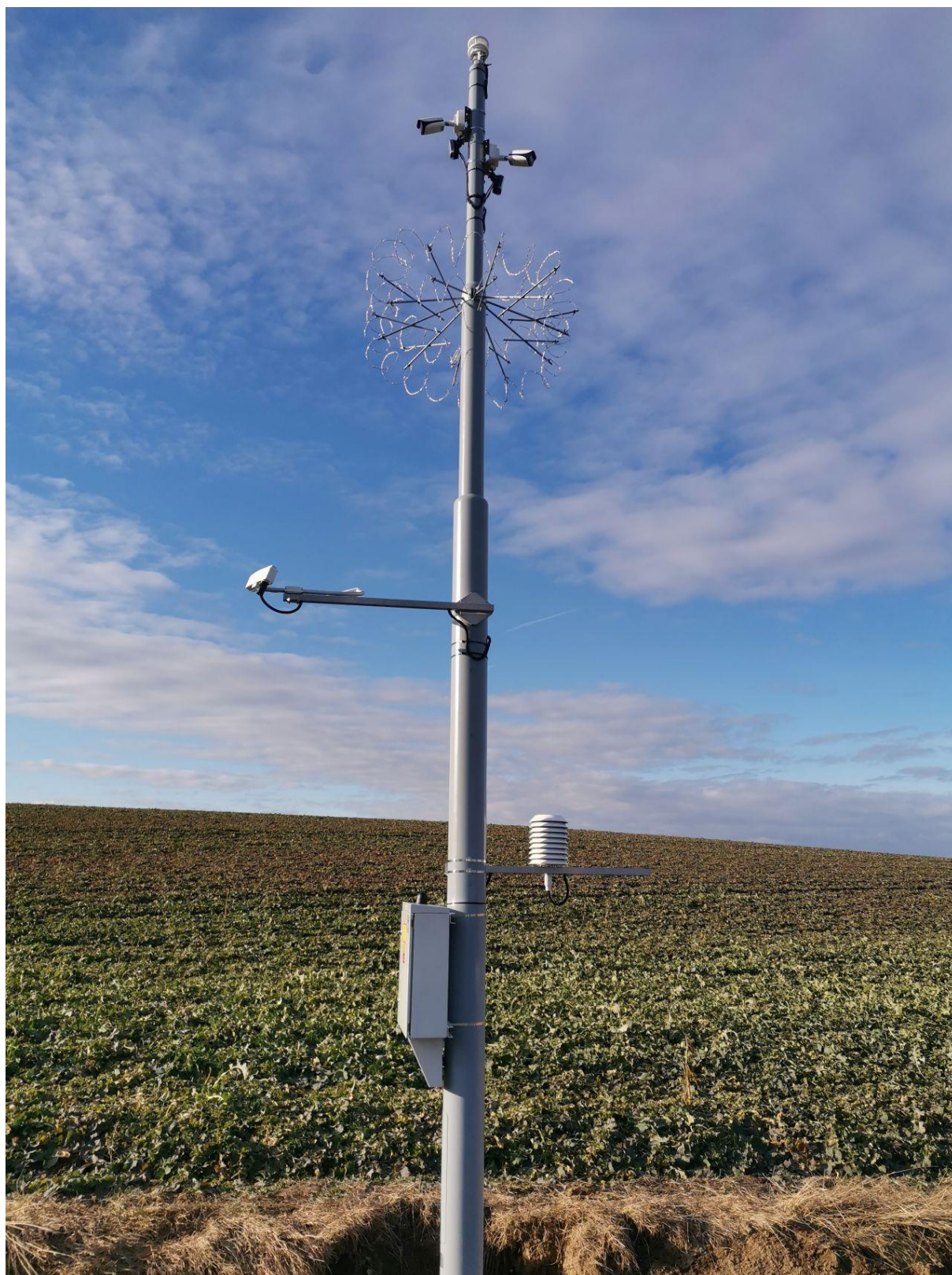
Fig. No. 14: Road meteorological station Rohov (Moravian-Silesian region)
