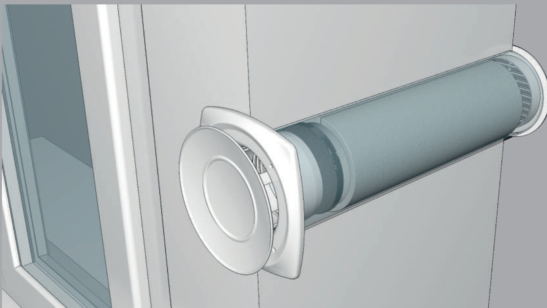
KP supply valve mounted in-walls.
