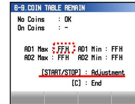
When AD1 MAX is smaller than 53H, Adjustment result is OK.
