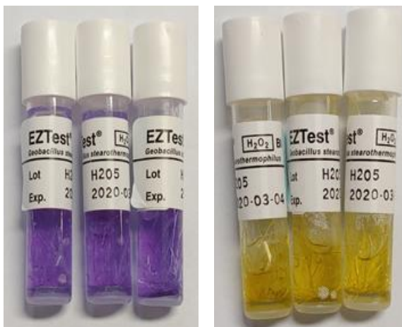
◀ BI Color change Successful sterilization(Purple), Failed Sterilization(Yellow)
