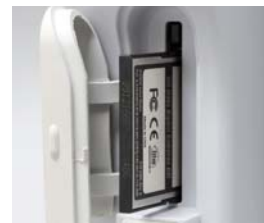
CF (Compact Flash) Media Card Slot The CF card allows direct recording of images during examination.
