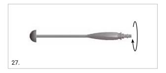
**Step 3:** Assemble the anvil and screw it until fully tightened.
