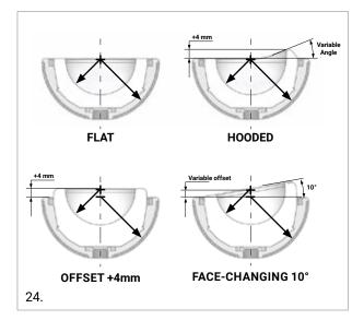
In the hooded liners, the hood makes an angle which is size dependant:
