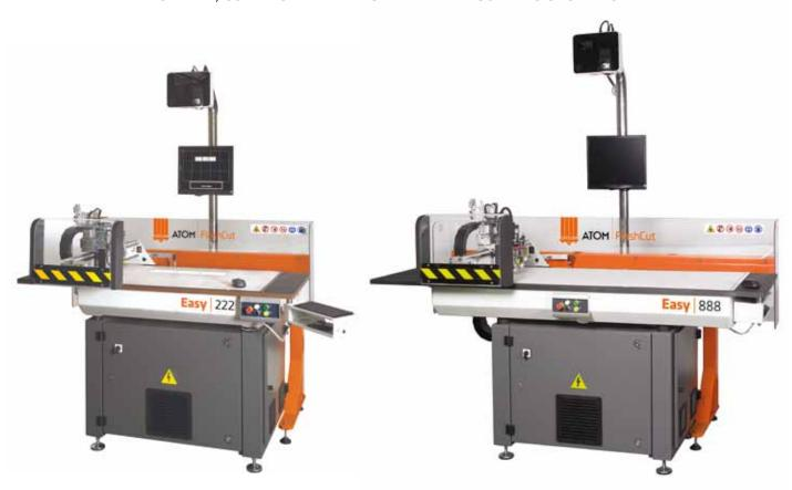
The FlashCut **Easy 222** and **Easy 888** perfectly meet the requests of footwear and leather goods industry. They represent the perfect choice for sample departments and small production batches. Their easy handling, flexibility and cutting accuracy are appreciated also for bigger productions. They can cut leather and hard leather for soles, as well as many man-made materials. Easy to use, they are the best choice for small companies or those who want to automate the cutting process.
