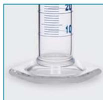
Hexagonal base with strengthened knobs ensures increased stability.
