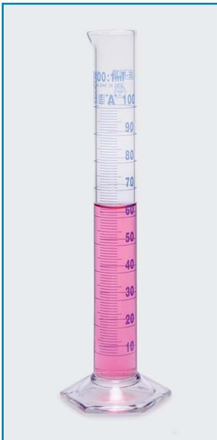
➤ Manufactured from heat resistant, durable borosilicate glass according to DIN EN ISO 4788 standard.
