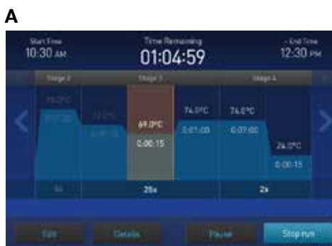
Figure 2. Graphical interface. Software allows (A) easy editing of thermal cycling conditions and viewing of plate layout, and (B) viewing of amplification plots and drilling down to a subset of sample wells.
