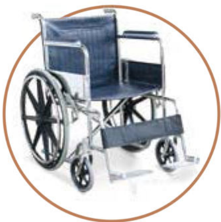
JL809B CHROMED STEEL FRAME, FIXED ARMREST, FIXED FOOTREST, SOLID CASTOR, SOLID REAR MAG WHEEL
