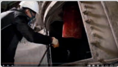
Application of mixer protection
