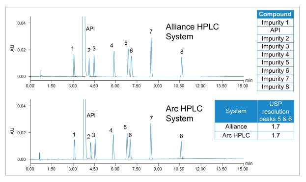
Figure 3. Comparison of chromatographic data for the analysis of an API and its impurities, demonstrating effective method transfer from an Alliance System to an Arc HPLC System. Analyses were performed using a CSH  $C_{18}$  Column (5  $\mu$ m, 4.6 x 150 mm). Mobile phase: 0.1% formic acid in water (A) and in methanol (B), at 2.9 mL/min; 10- $\mu$ L injection volume and passive pre-heater installed in both systems.
