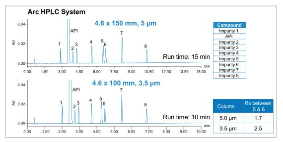
Figure 6. Comparison of chromatographic data for the analysis of an API and its impurities demonstrating successful scaling of the original method from a CSH  $C_{18}$  Column (5  $\mu$ m, 4.6 x 150 mm) at 2.9 mL/min with a 10- $\mu$ L injection to a CSH  $C_{18}$  Column (3.5  $\mu$ m, 4.6 x 100 mm) at 2.3 mL/min with a 6.7- $\mu$ L injection. Analysis condition: mobile phase, 0.1% formic acid in water (A) and in methanol (B).
