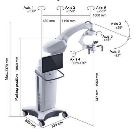
Figure 90: Dimension diagram
