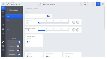
*Figure 86: "Settings Microscope" menu, "Light" submenu for the LED light source*
