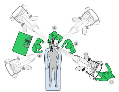
Figure 77: Possible positions for cranial procedures and ENT
