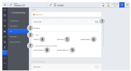
Figure 42: "Settings Connectivity" menu, submenu: "LAN"
