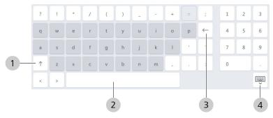
Figure 11: Screen keyboard key assignment
