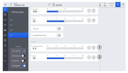
Figure 28: "Settings Microscope" menu, "Zoom" submenu
