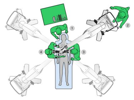
*Figure 78: Possible positions for face-to-face procedures, e.g. spine procedures and P&R surgery*
