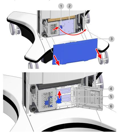
Figure 88: Changing the lamp on the light source
