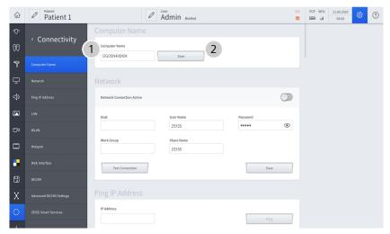
Figure 47: "Settings Connectivity" menu, submenu: "Computer Name"
