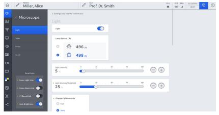
*Figure 85: "Settings Microscope" menu, "Light" submenu for the xenon light source*
