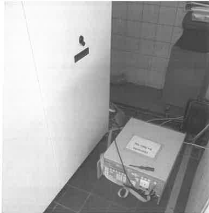
Photo of test setup for Electrical Fast Transients
