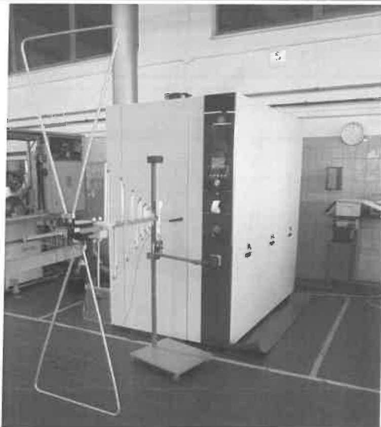
Photo of test setup for Radio Frequency Electromagnetic Fields
