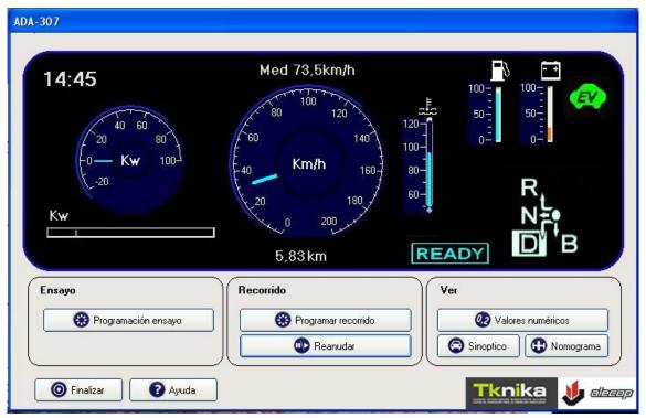
The hardware trainer is a driving simulator (gear, speed, battery charge, fuel gauge). All the actions performed on the panel are represented in the software instrument panel. The ADA307 software provides information on vehicle performance in figures, graphics, and gauges. The user can choose to view the numerical data screen, the nomogram screen, or the synoptic chart screen.
