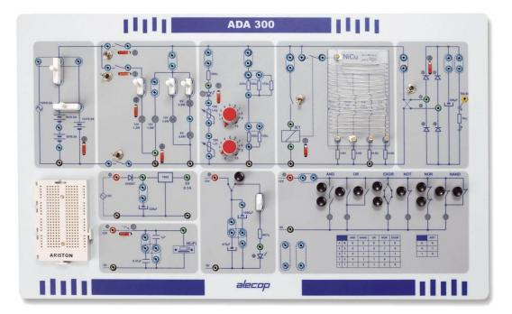
The purpose of this equipment ADA300 is to familiarise students, in a flexible way, with basic electricity in general and more specifically its application in cars. The application can be used to analyse and check different basic electric circuits as well as their components without wasting any time on assembly and dismantling.
