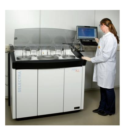
With random access and typical throughput of 400 tests per hour, the Selectra ProXL System is a compact, self-contained floor standing solution for primary, STAT or back-up testing. This new system offers minimal maintenance and efficient use of consumables to truly reduce operational cost.
