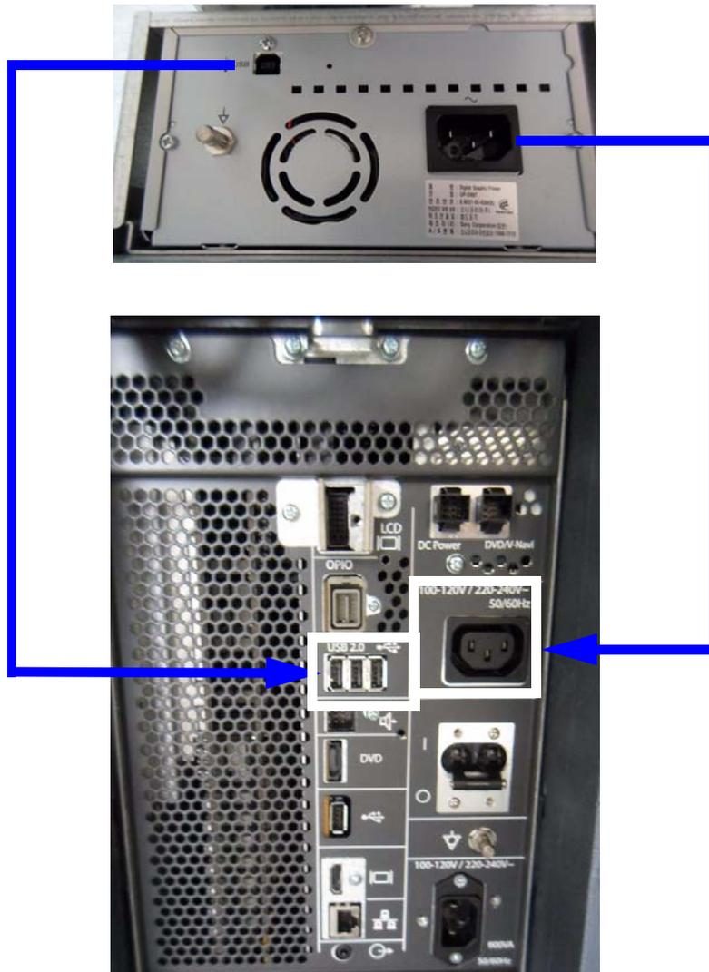
Figure 3-37 R1 and R2 Black & White Printer connection
