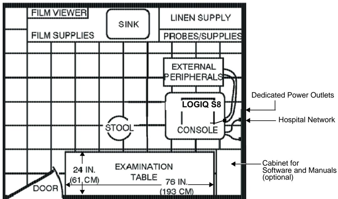
Figure 2-1 Minimal Floor Plan 4.3m x 5.2m (14ft x 17ft)
