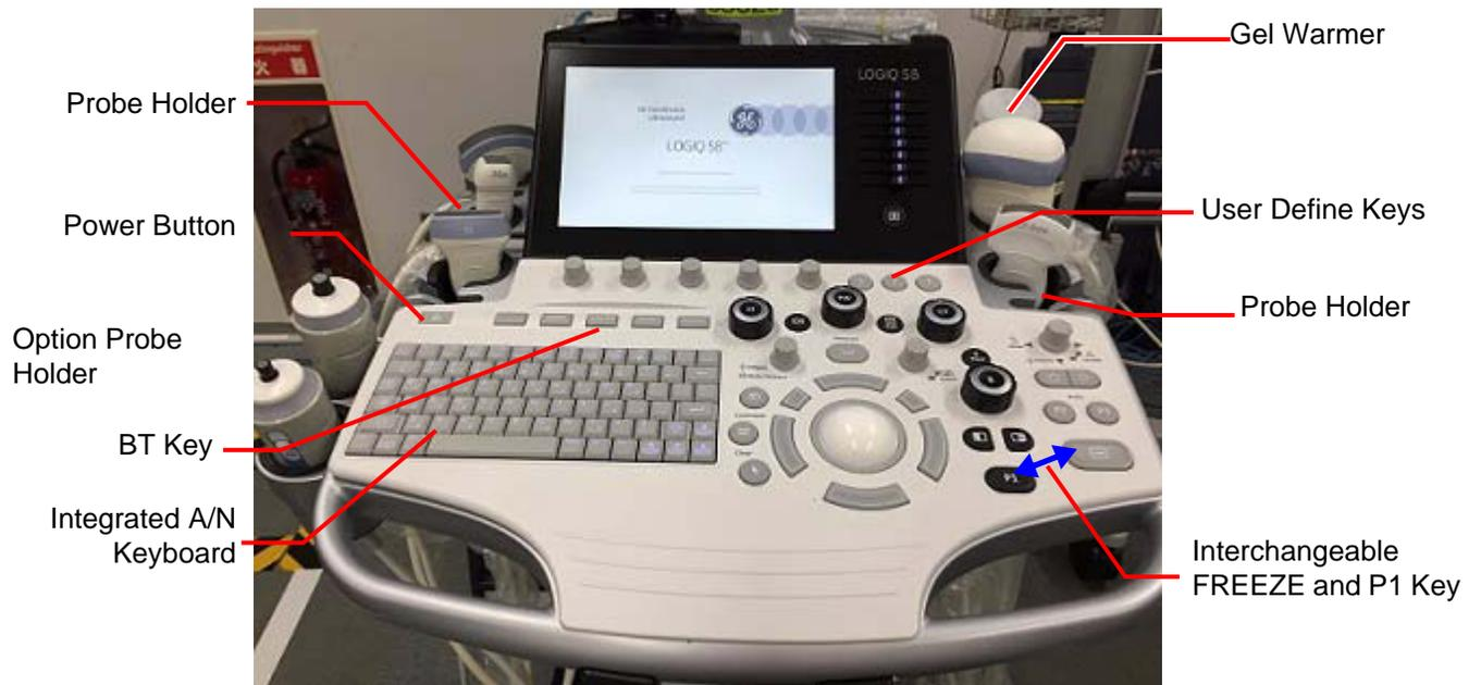
Figure 5-4 R4 and later Operator Panel
