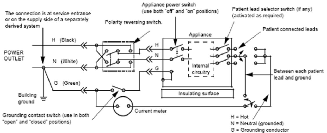
Figure 9-8 Test Circuit for Measuring Patient Lead Leakage
