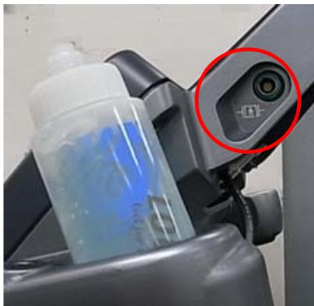
Figure 3-34 ECG Connector location (R1 to R3 system)
