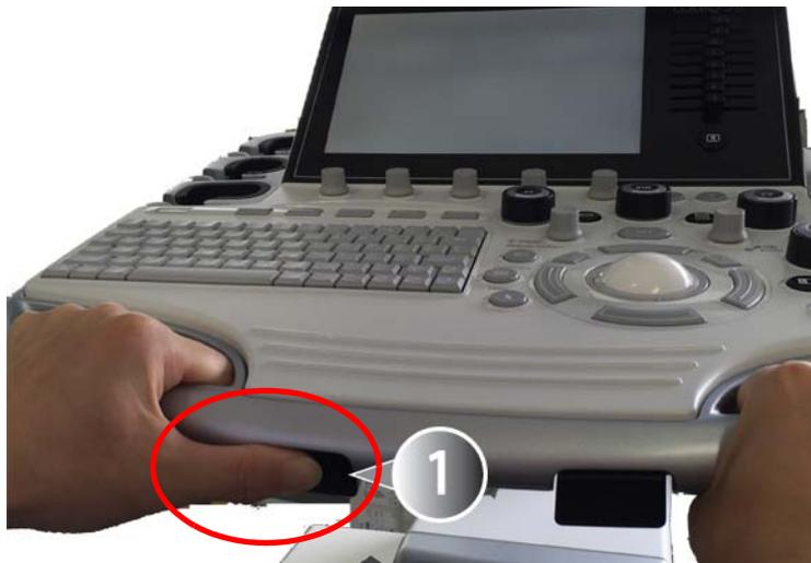
Figure 4-8 Swivel Lock Lever (R4 system)
