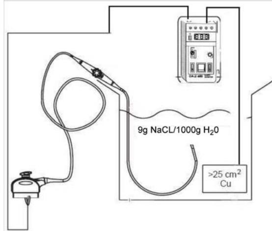
Figure 9-14 TEE Probe Leakage Isolation (Sink) Current Test
