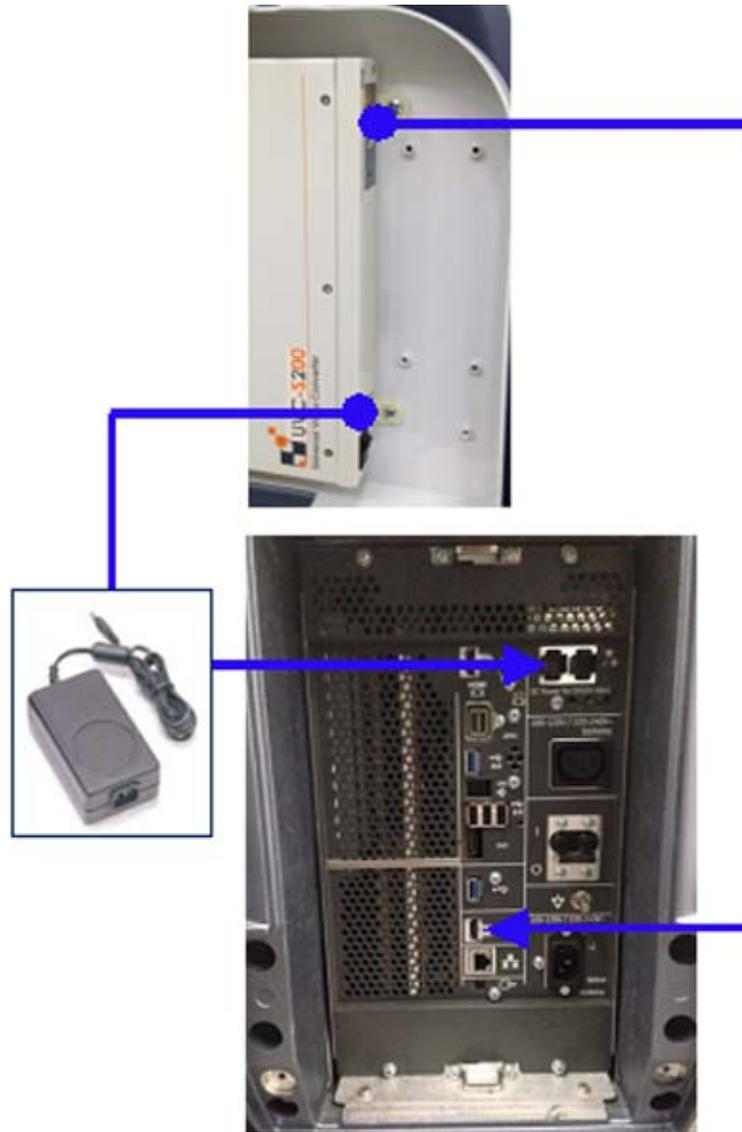
Figure 3-32 On-Board UVC Connection for R3 and later
