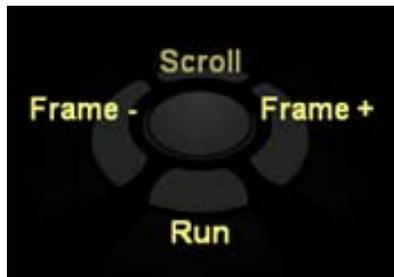
Figure 4-17 Example: Trackball key Function
