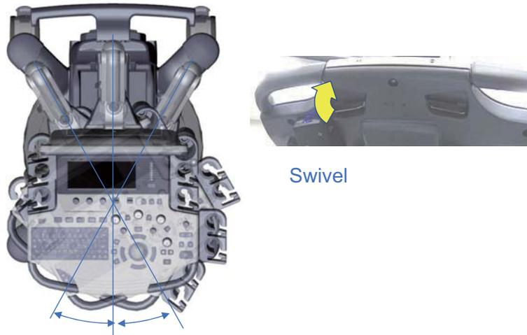
Figure 4-7 Swivel Lock Lever (R1 - R3 system)
