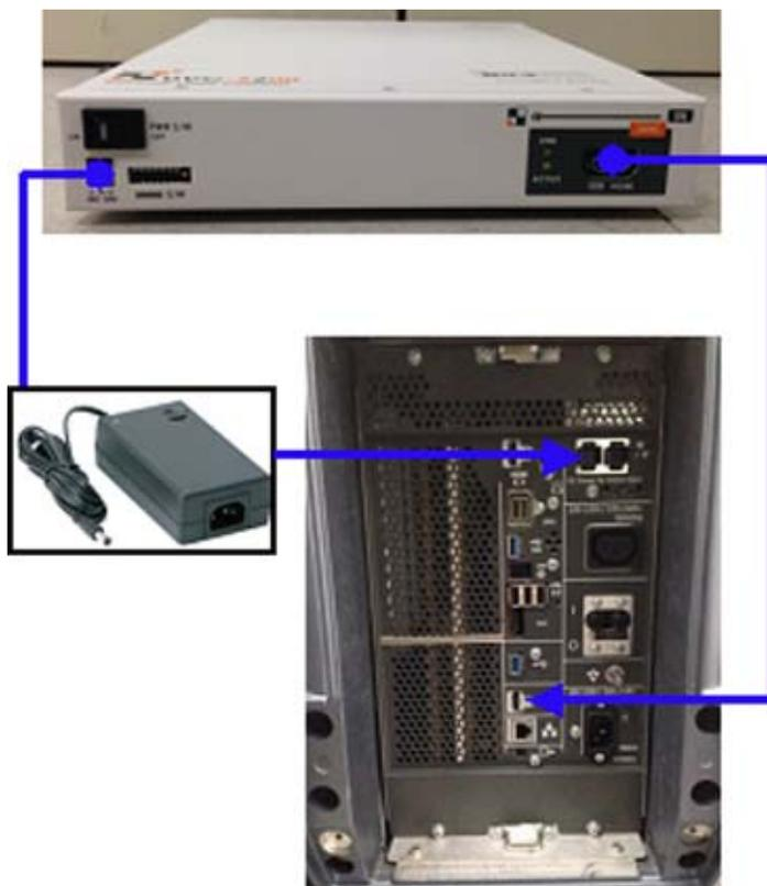
Figure 3-30 Off-Board UVC Connection for R3 and later
