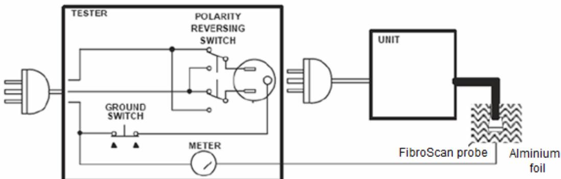
Figure 9-10 Set Up for FibroScan Probe Leakage Current
