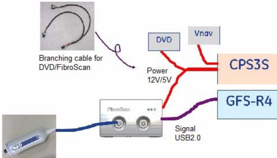
Figure 5-13 Signal Connection
