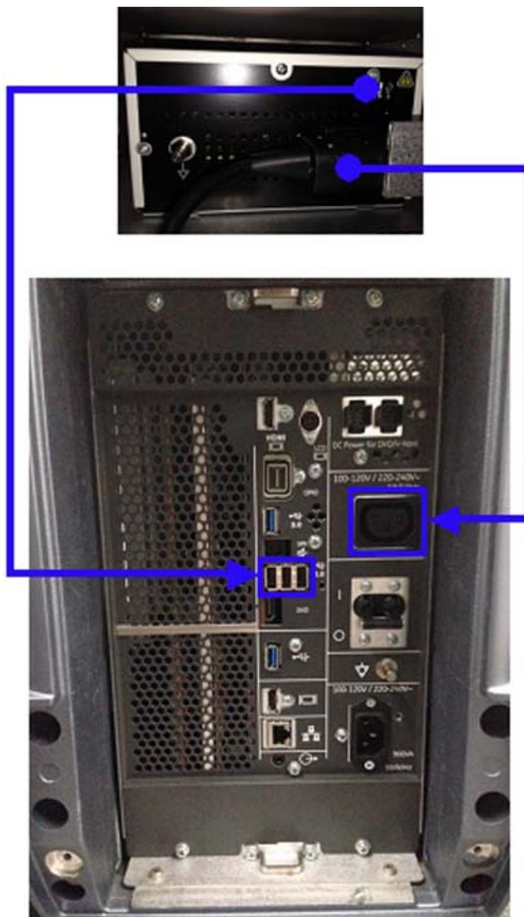
Figure 3-38 Black & White Printer connection for R3 and later
