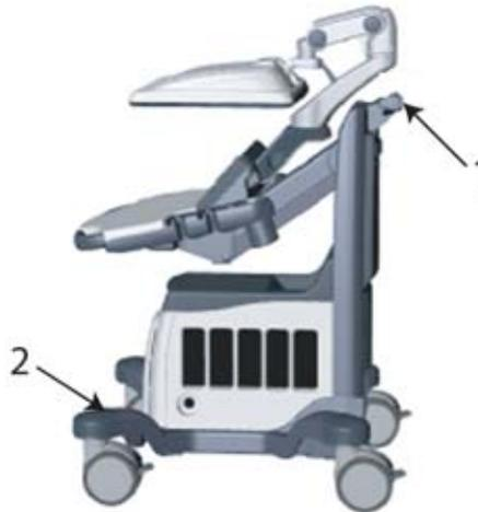
Figure 4-13 Wrapping position of the belt
