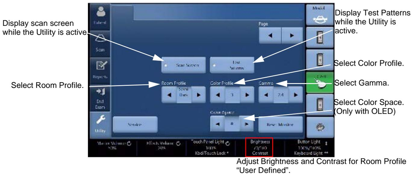
Figure 6-7 Utility second page - 22" OLED Monitor example
