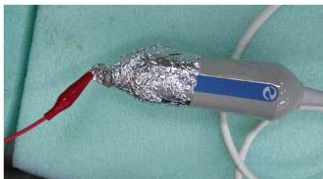
Figure 9-12 FibroScan probe with Aluminium foil
