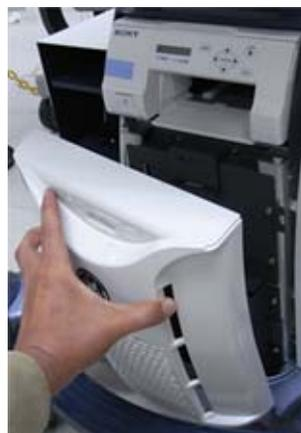
Figure 9-2 Remove the front cover
