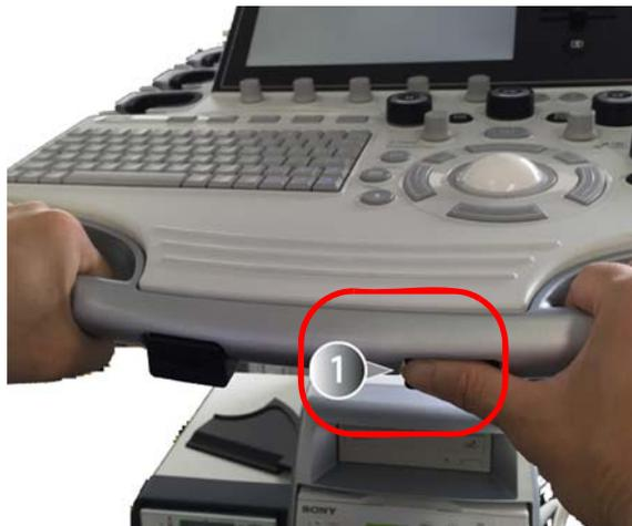
Figure 4-6 Elevation Lock Lever (R1 - R3 System)
