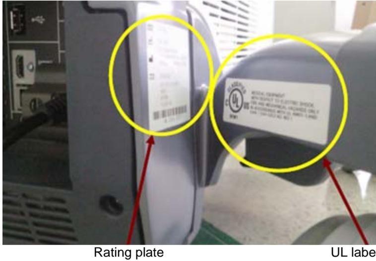
Figure 1-5 Rating plate and UL label - example
