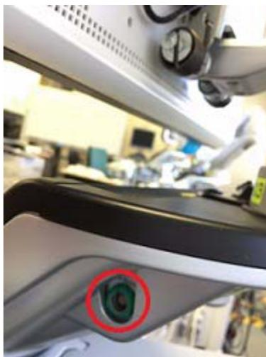
Figure 3-35 ECG Connector location (R4 system)
