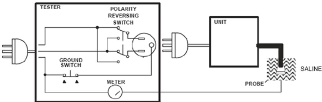
Figure 9-9 Set Up for Probe Leakage Current
