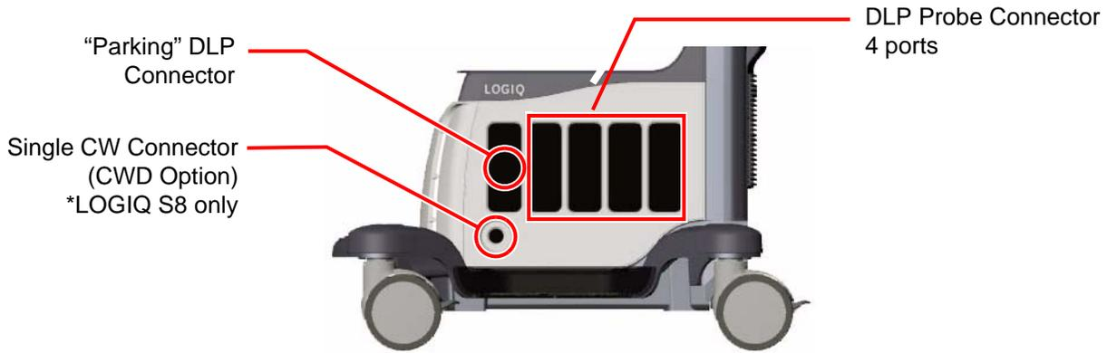
Figure 5-5 Probe connector
