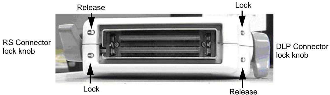
Figure 3-9 Lock/Release position
