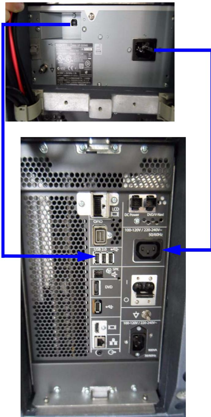
Figure 3-40 R1 and R2 Color Printer connection
