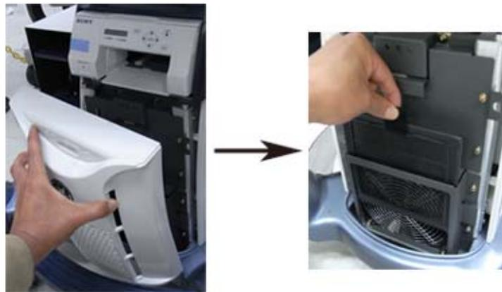
Figure 9-1 Air filter location
