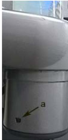
Figure 4-29 Gel warmer ON/OFF switch
