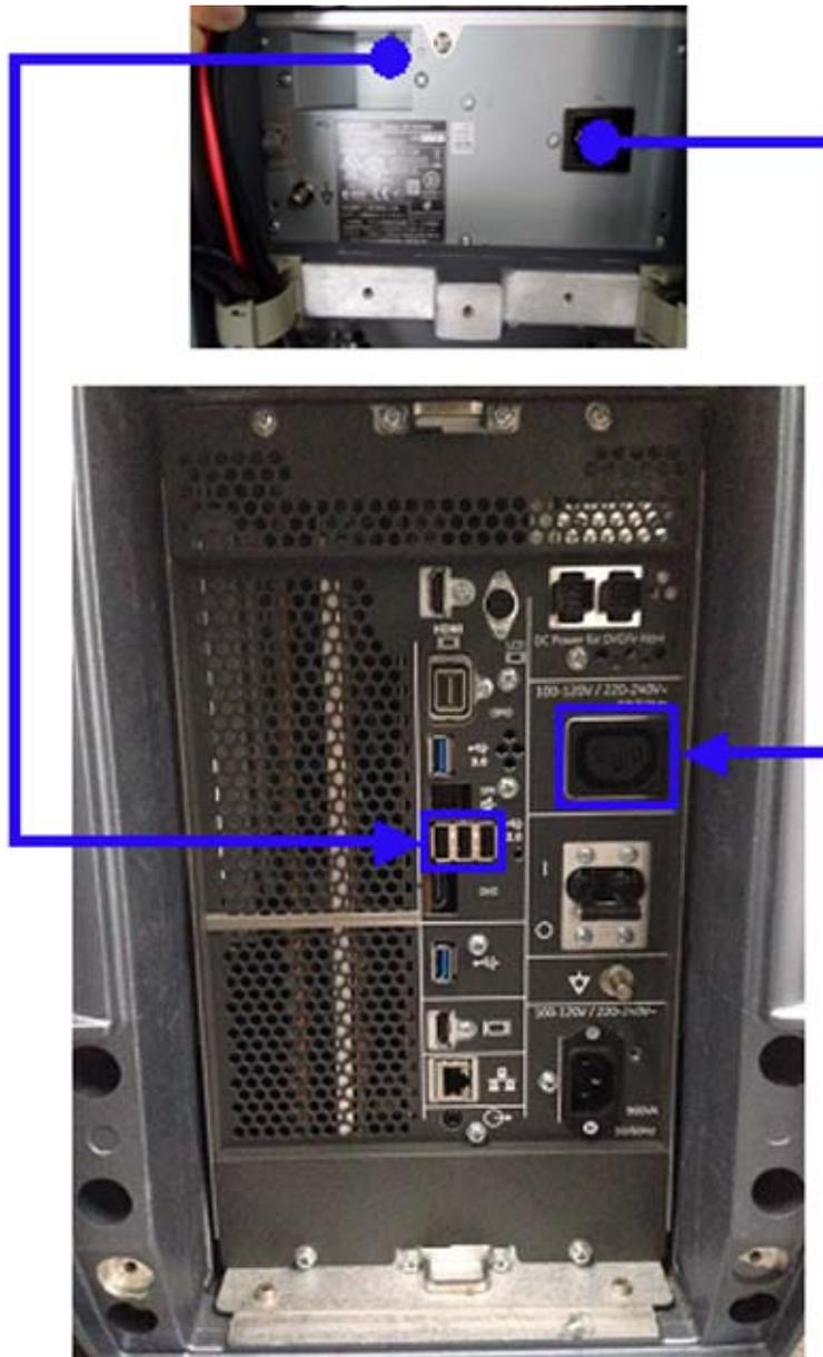
Figure 3-41 Color Printer connection for R3 and later
