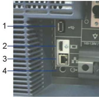
Figure 3-6 External I/O Connectors - on Rear of System
