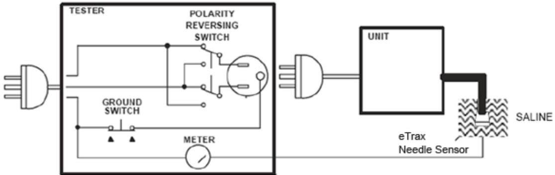
Figure 9-15 Set Up for e-TRAX Leakage Current
