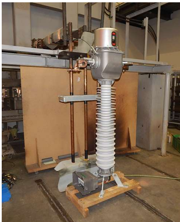
Short circuit withstand capability test
