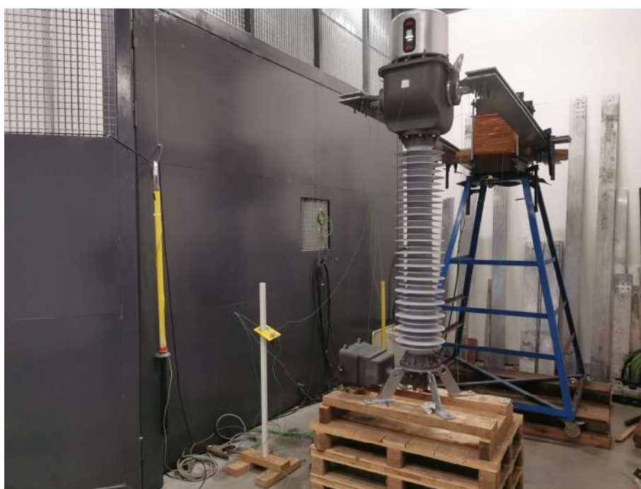
Temperature rise test
