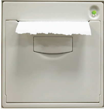
Figure 2-10 Installing Thermal Paper (3)
