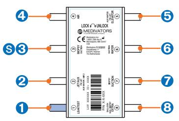
Each Hookup is comprised of multiple ports and connector assemblies. Each port is labeled with a Port ID number (circled). This same number also identifies the corresponding Connector Assembly. Each Connector Assembly is fitted with a specific endoscope connector.
