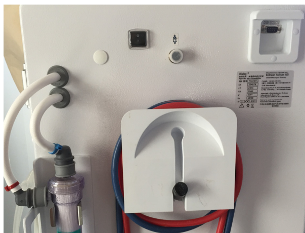
Fig. 4-1 Storage of cables and tubes
