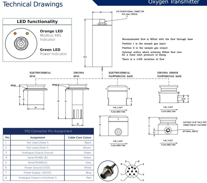
Notes: 1. Cable cores that are not used must be insulated / heat-shrinked.
