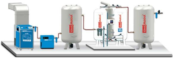
Fig. 1: Structure of the Oxygen Generator System
