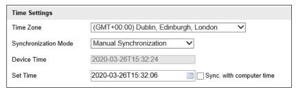
Figure 6-8 Manual Synchronization
