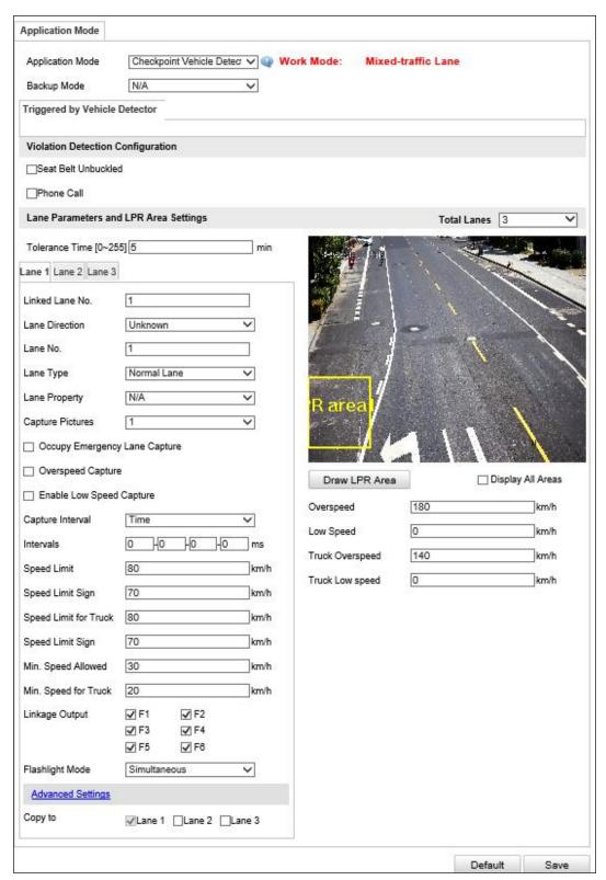
Figure 11-15 Checkpoint Vehicle Detector
