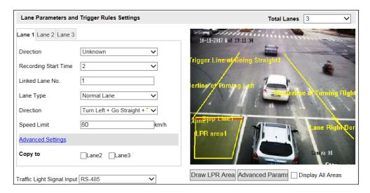
Figure 11-5 Lane Parameters and Trigger Rules Configuration
