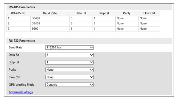
Figure 6-2 Serial Ports Settings
