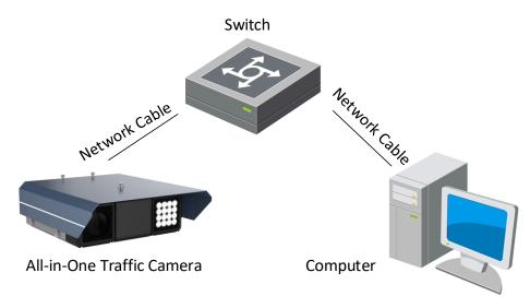
Figure 1-2 Connecting via a Switch or a Router
