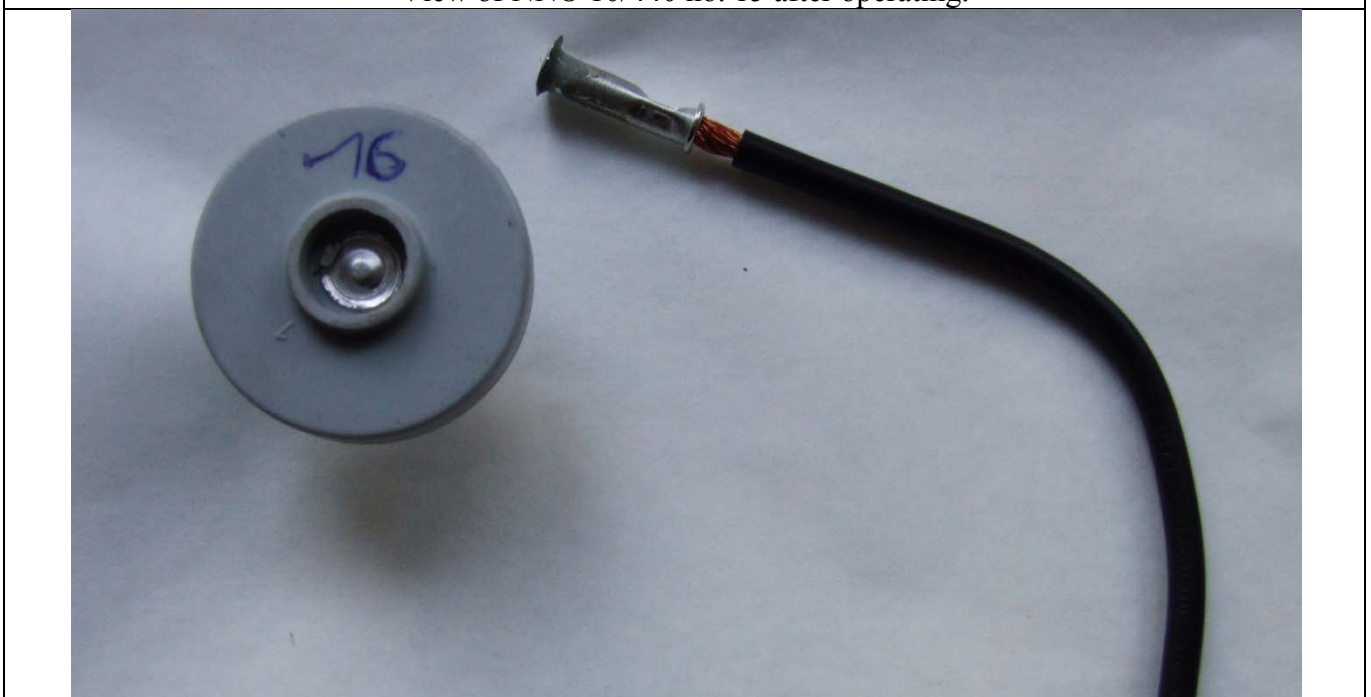
View of NNO 10/440 no. 16 after operating.
