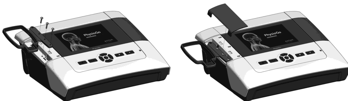
Figure 4.6. Sample view of mounting the holder for cluster laser applicator
