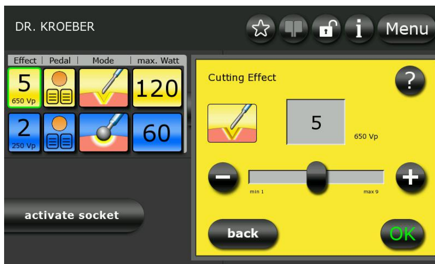
Figure 5-10: Effect monopolar cutting
