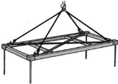
Example of container lifting using a lifting beam fitted with hooks, shackles or manually coupled lock
