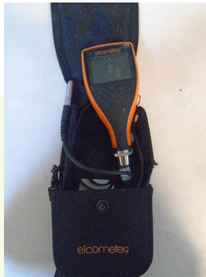
Figure 9: Elcometer Used for Coating Thickness Measurement (Date of test: 25-November-2024)
