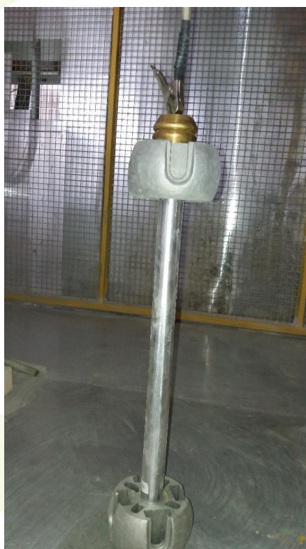
Figure 8: Brass Electrodes Used in Water Diffusion Test (Date of test: 02-December-2024)
