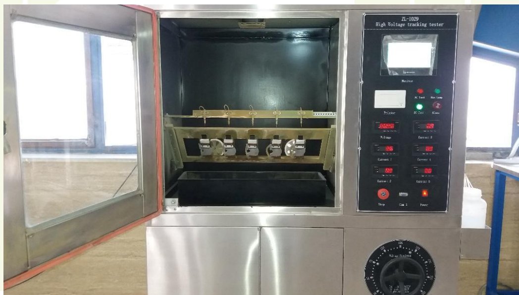
Figure 6: Tracking Machine Tester (Date of test: 26-November-2024)
