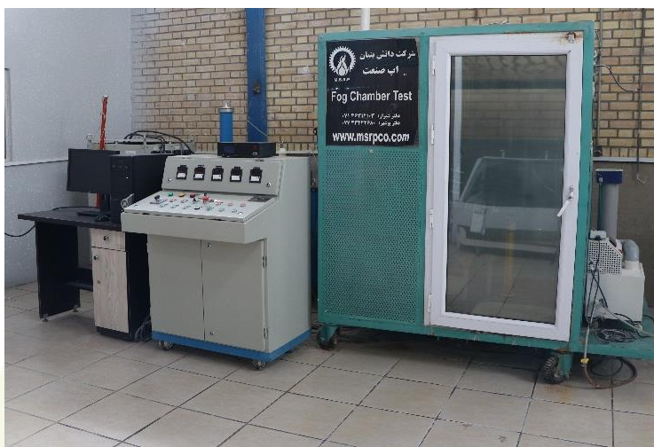
Figure 15: Salt fog Test Machine (Date of test: 14-December-2024)
