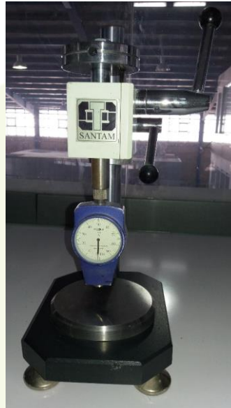
Figure 5: Shore A Durometer (Date of test: 27-November-2024)
