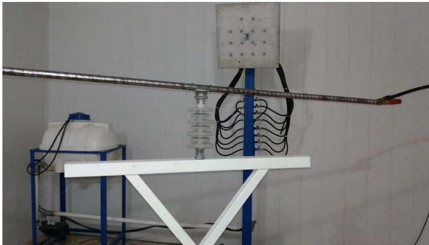
Figure 11: Wet Power Frequency Voltage Test Chamber (Date of test: 26-November-2024)
