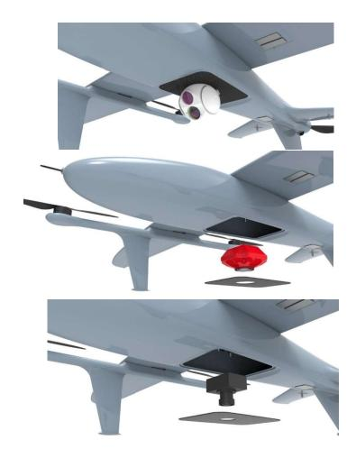
380 "humpbackwhale" VTOL UAV can carry various payload such as EO/IR pod, Orthophoto camera and etc., and be applied to security surveillance, patrol reconnaissance, geographic mapping and surveying, powerline inspection and other fields.
