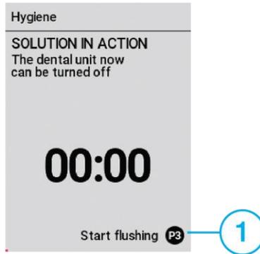
5. TO START FLUSHING – By starting the flushing, the screen for setting the flushing time is displayed.
