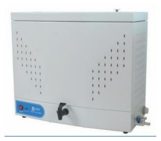
Stainless steel water still for automatic and continuous operation with built-in 8/16 I storage tank. For bench and wall mounting. Supplied with wall mounting bracket. Excellent quality of distillation. An electronic level switch switches the still off when the storage tank is full and restarts it automatically when destilled water is withdrawn. Dispenser Tap of distilled water. With flow regulator to avoid excessive water consumption.
