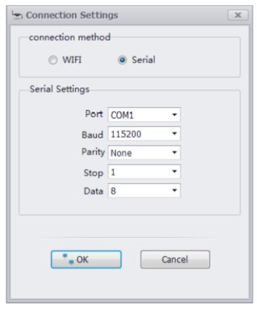
Figure 4-7 Device Connection Settings
