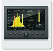
Loudness Radar Meter; a state-of-the-art true peak meter; downmix compliance; stereo correlation; and a RTA (Real Time Analyzer).
