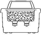
During the low pressure stage, millions of microscopic bubbles form and grow. This process is called CAVITATION, meaning "formation of cavities".
