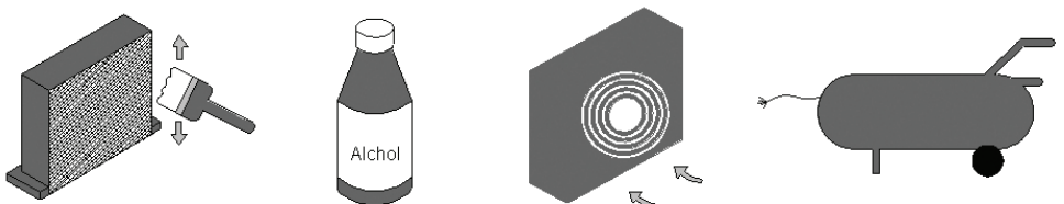
Figure 6 Cleaning of the Condenser
