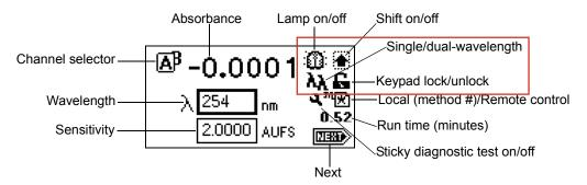
You can recall the absorbance screen at any time by pressing the HOME key. When you first use of the detector, the absorbance screen shows the factory-set defaults. Afterward, the absorbance screen shows the settings displayed before the detector was last powered-off. The absorbance screen continues to change as the run continues.
