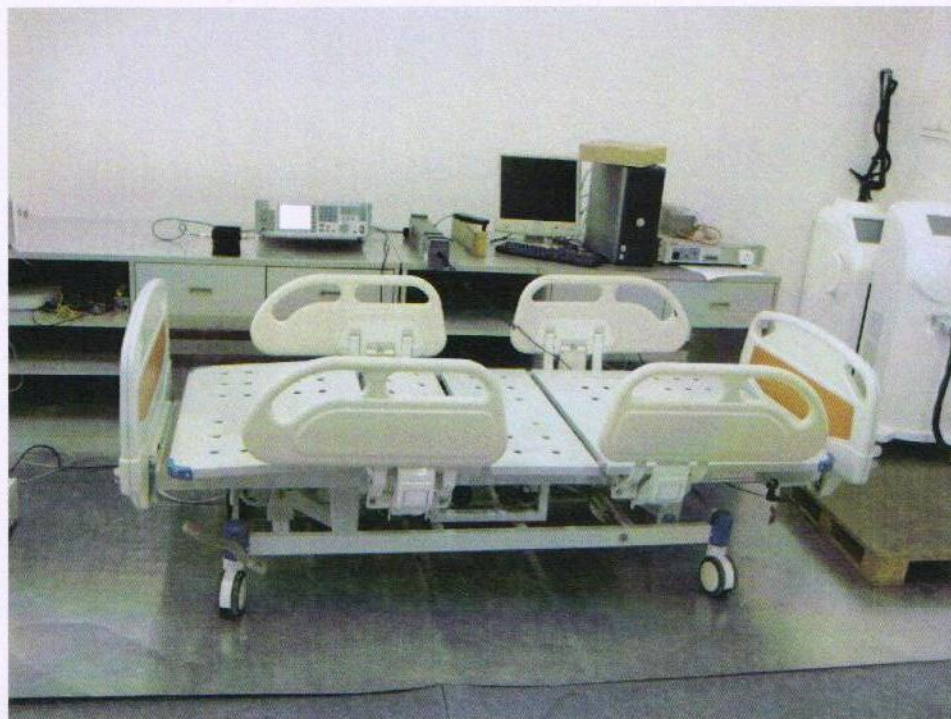
Photograph 8: Set-up for immunity test of injected current, signal line
