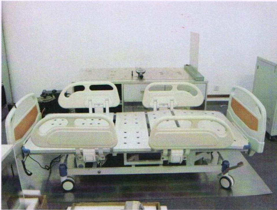
Photograph 4: Set-up for immunity test of RF electromagnetic field, 80M-1GHz
