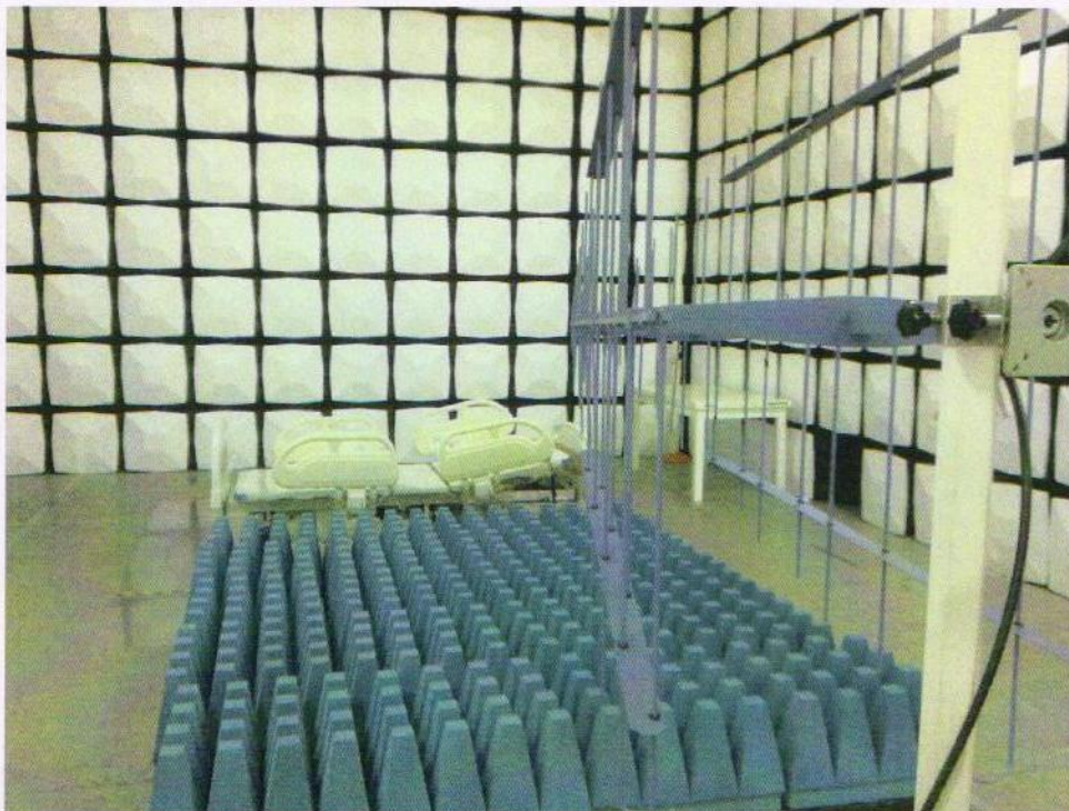
Photograph 4: Set-up for immunity test of RF electromagnetic field, 80M-1GHz
