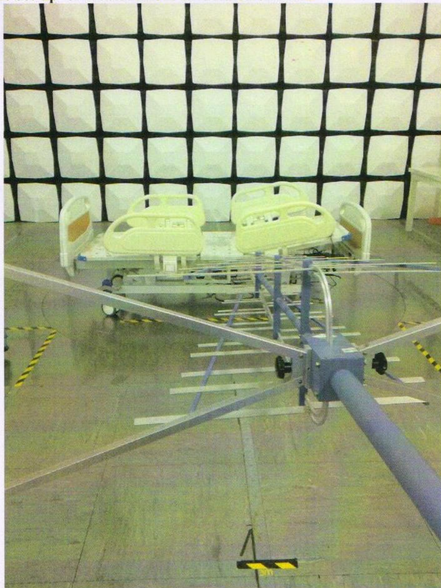
Photograph 2: Set-up for measurement of radiated emission
