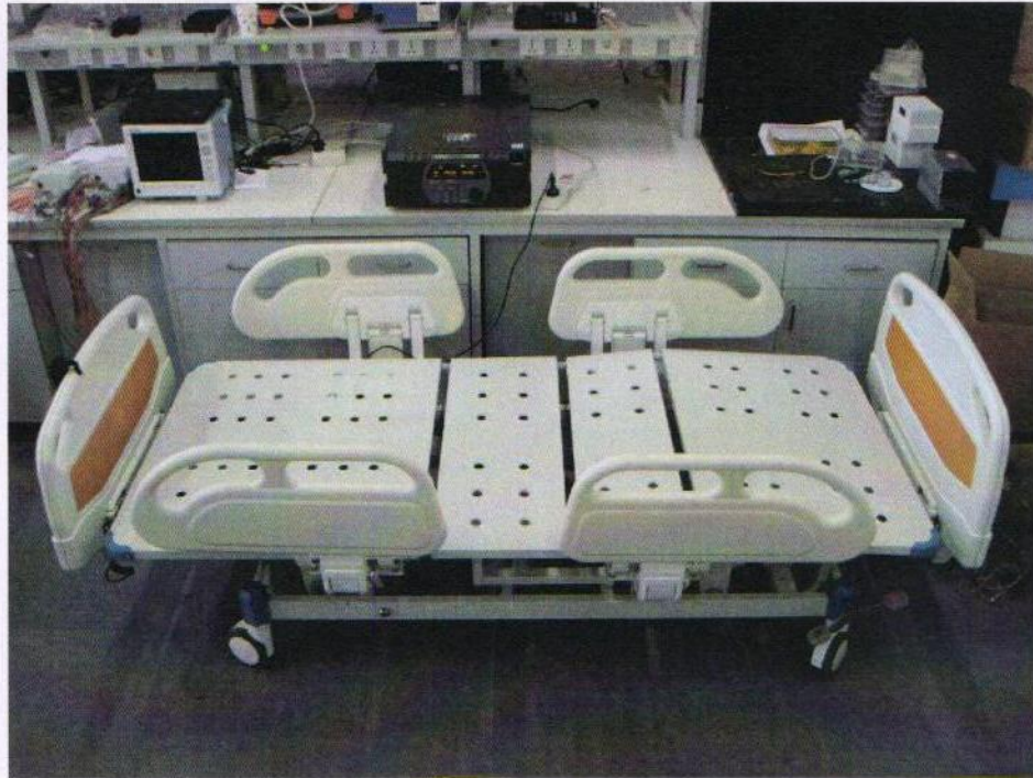
Photograph 10: Set-up for harmonics on AC mains
