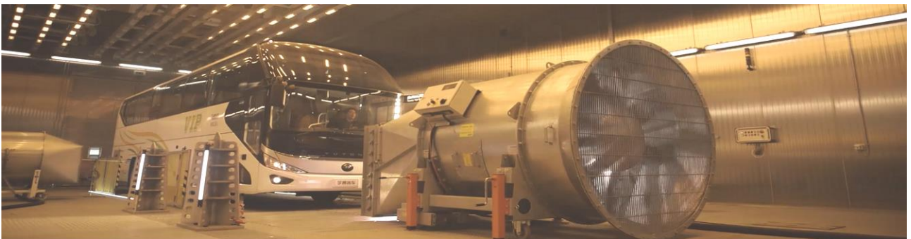
Simulation Test Cabin of Vehicle in High-low Temperature Environment of German ENGIE Company
