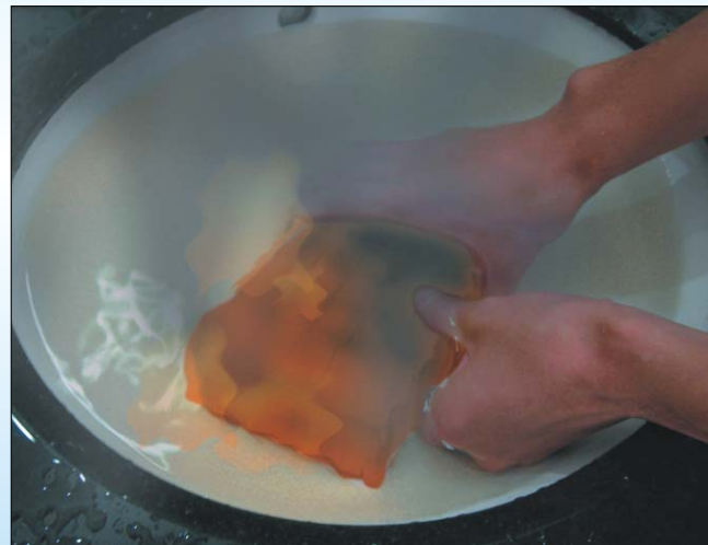
將冒烟燃燒的電池浸入水中 Put the burning battery into water
