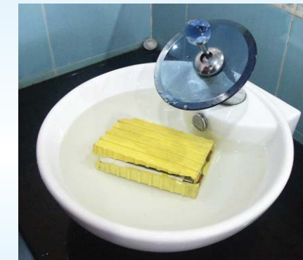
將裸露的電池泡入水中 Put the uncovered cell into water
