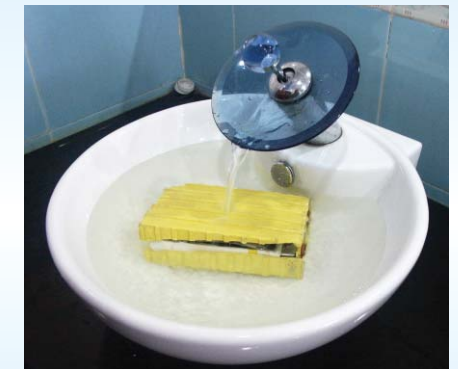
裸露的電池被水完全浸泡 Uncovered cell gets fully soaked by water
