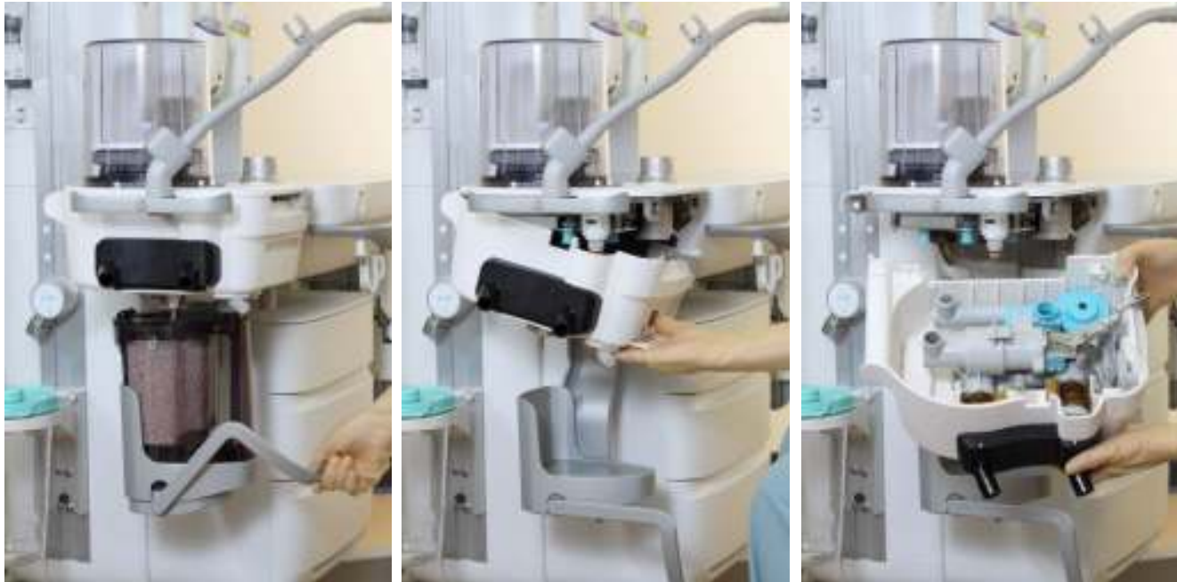
Step 1: remove CO2 absorber Step 2: unlatch breathing circuit Step 3: remove breathing circuit
