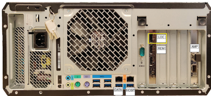
Figure 7. Local Monitor Display Connection.
