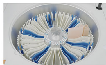
Reagent Tray 2~8°C cooling for 24 hours.
