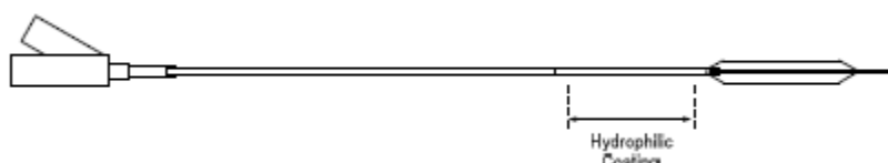
Fig. 1: Schematic drawing of the FREEWAY™ 035 Paclitaxel eluting PTA balloon catheter.
